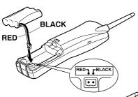
2 Connect the battery pack connector with the correct polarity (black and red wires), then insert the battery pack into the battery compartment.
