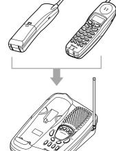
4 Place the handset in the base unit with the keys and display facing upward. This position lets you see Caller ID messages on the display.
